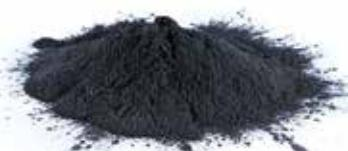
BESLEYEN K is exothermic mouldable feeder compound can be moulded into convenient shapes such as hollow cylinders or sleeves by means of its binding type agents and inserted in the riser cavities.
