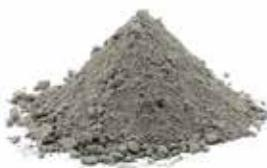
Exothermic hot topping compounds support feeder functionality. These exothermic materials has low-emission parameters, assist in feeding systems and advantage of high-flexible usage.
